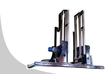
2-axis robotic MANIPULATOR with dedicated extraction PLATE for horizontal / vertical
